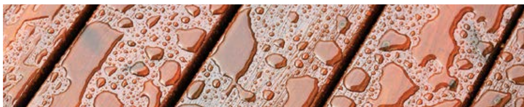
Figure 8: Filler surface treatment
