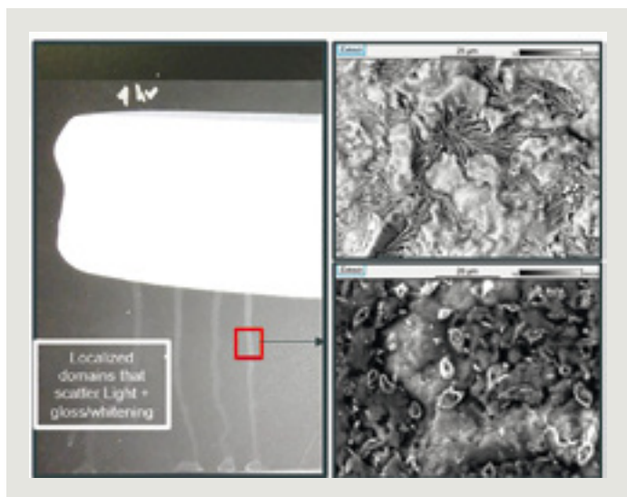
Figure 2: Left: optical image showing snail trails from a white paint onto a black substrate. Right: Scanning electron micrographs showing two different types of crystal formation.
